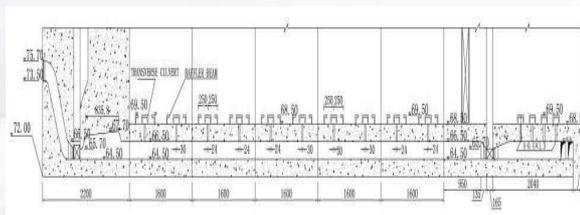
Longitudinal Culverts Under the Lock Floor (Fig. 4.18)
