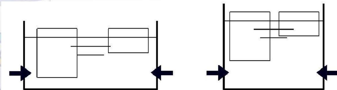
Impact of the wall culvert side port system (bad configuration on the left, better one on the right) (Fig. 4.23)
