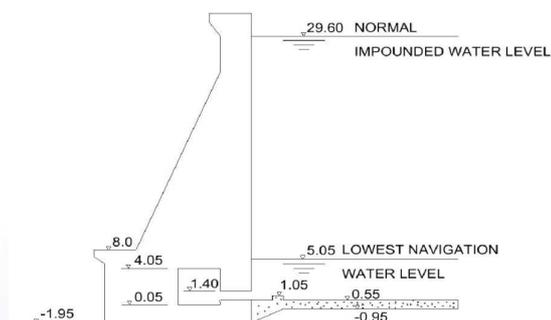
Wall Culvert Side Port System (Fig. 4.13)
